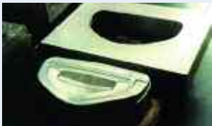
Punch and blankholder finished.
