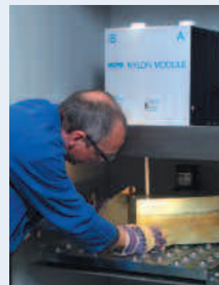
Load the silicone mould. Standard silicone mould technology is used for this process.
