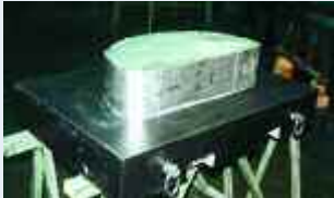
To produce the punch, fill the casting pattern with MCP Alloy using a pre-prepared sheet metal retainer frame.
