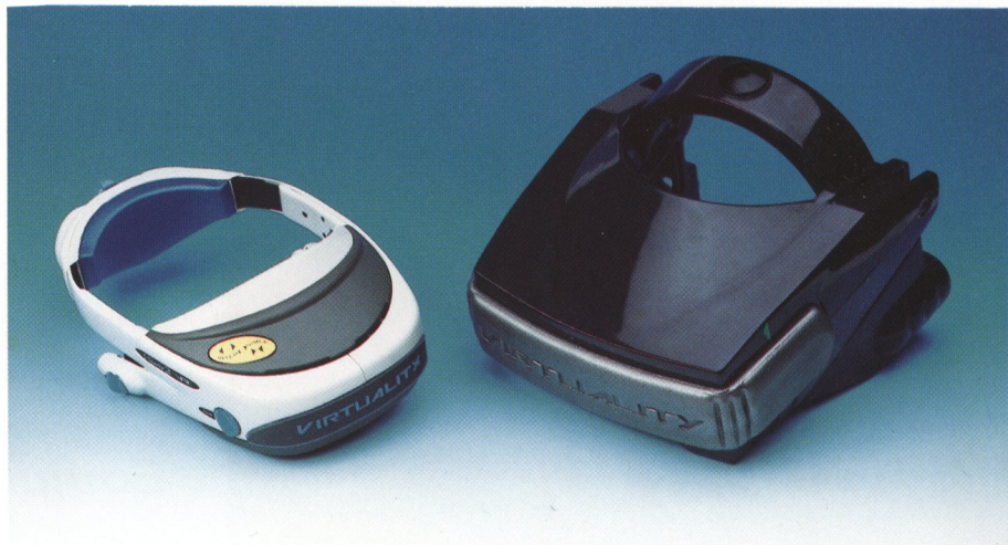
Virtual-Reality Visers produced with the MCP Vacuum Casting Process. The visers consist of up to seven different vacuum plastics ranging from very soft 40 Shore A to ABS-like materials. The models were produced by Rapid Prototyping
