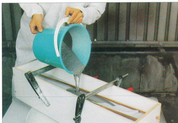
Back-up the metal sprayed shell with high temp resin
