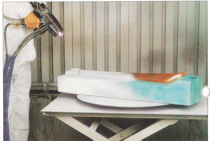
Cool spray the model with MCP/TAF moldmaking wire. 8830 type gun.
