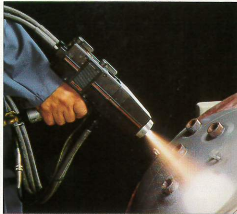
High temp spraying with the 8830 gun. MCP has ongoing development to create new mold surfaces to satisfy customer needs
