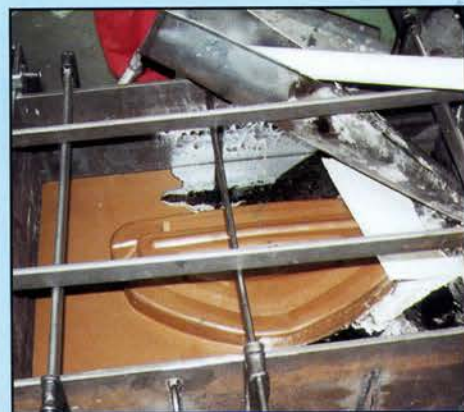
...and cast the MCP Alloy to produce the bottom die.
