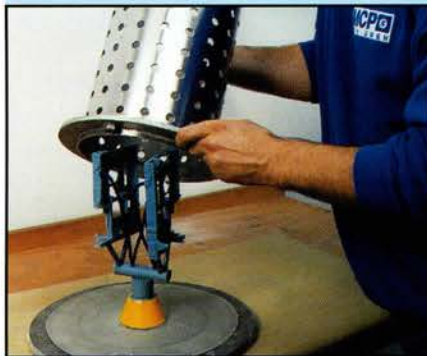
2. Place the casting flask over the wax models.
