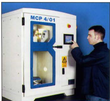
New: Produce wax components for metal part casting (lost wax process)
