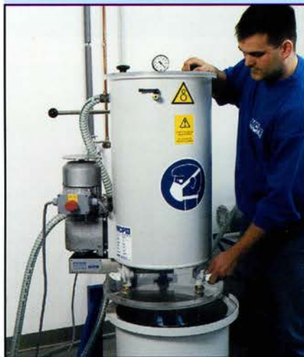
3. Mix and cast ceramic under vacuum to encapsulate the wax models in the flask. Place in the oven.
