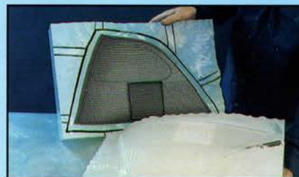
4. Revealing the master model faithfully reproduced in the silicone. The master model is then removed.
