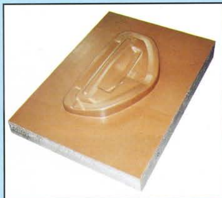
Coat with wax sheet in the thickness of the sheet metal to be used...
