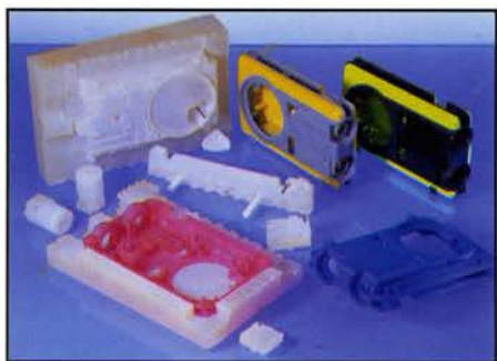
New: Produce wax components for metal part casting (lost wax process)
