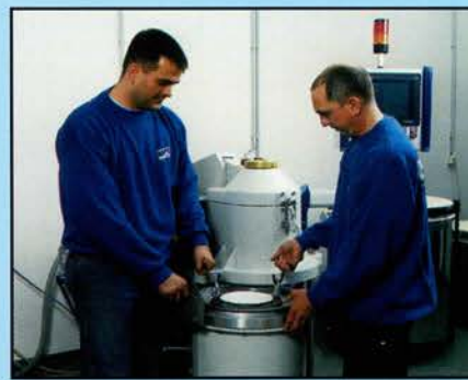
4. Remove the flask from the oven and place into the casting unit and close.
