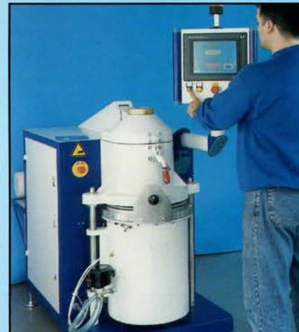
5. The PLC touch screen controller will operate all important parameters of the casting process. Melting takes between 15 and 20 minutes depending on the type and amount of metals. The casting operation is performed automatically in just a few seconds giving perfect results. No heat radiation, no dirt, no fumes..
