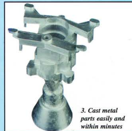
6. The metal part can be removed from the ceramic mold within 30 to 60 minutes after casting.
