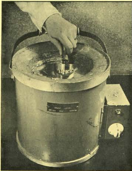
Fig. 9.—Producing Cerrotru dip-cast mould on metal master pattern.
